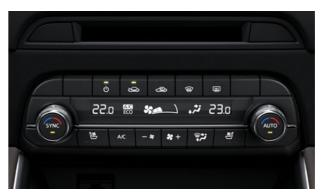
The climate-control system with full-auto air conditioner gives excellent heating/cooling performance with low energy consumption. Its control panel layout features a horizontal orientation to match the overall interior design.
