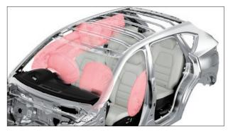
A full complement of airbags - front, front seat side, curtain provide another layer of protection in depth against physical shock and injury in a collision.
