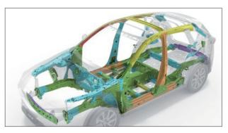
The body provides excellent collision safety performance. Extensive use of ultra-high-tensile steel gives strength with low weight, while the framework absorbs and channels energy away from the cabin.
