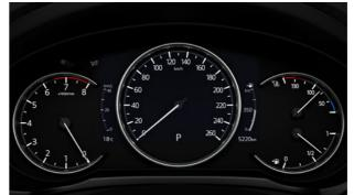
The three-meter cluster features a seven-inch TFT LCD colour display in the centre. In addition to vehicle speed, it shows diversified vehicle information in a clear, easy-to-read manner near the centre of the driver's line of sight.
