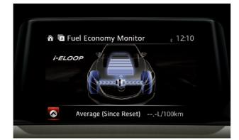
Mazda's i-stop idling stop system automatically shuts the engine down when you halt after braking. And the i-ELOOP regenerative braking system captures energy lost during deceleration, saving it as electrical power. Both technologies contribute to Mazda3's excellent fuel economy.
